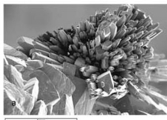
2. Fibrous-radial aragonite needle aggregate (SEM image). b) Eccentric aragonite stalactites.
